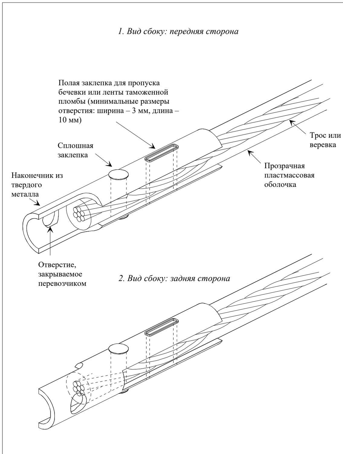
**Рисунок 6****ОБРАЗЕЦ СИСТЕМЫ КРЕПЛЕНИЯ БРЕЗЕНТА**
